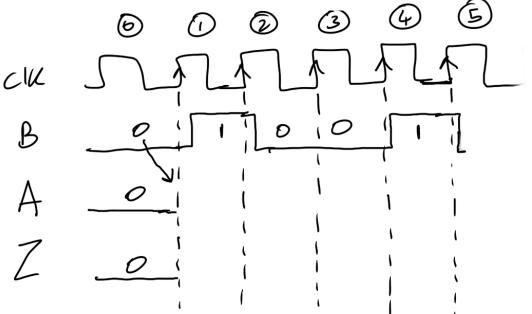
2. Create a Finite State Machine to handle the following requirements. There is an input A that is 0 or 1. The output Z should be set to 1 if A goes through a sequence of 1->0->1. So if A is 1 in cycle 1, 0 in cycle 2, 1 in cycle 3, Z should go to 1 for cycle 3. And if A goes to 0 in cycle 4 and A goes to 1 in cycle 5, Z should go to 1 for cycle 5 as well because cycle 3,4,5 have a sequence of 1->0->1.
